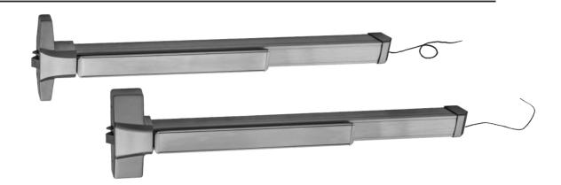
The Electric Latch Retraction (ELR) feature provides a remote means of unlocking exit device, once the latch bolt(s) retracted, the exit door is immediately changed to a push -pull operation. It is used for high security exit doors that require access control, or any room and place which needs quiet operation for opening the door such as conference rooms, libraries, hospital operating rooms, movie theaters, etc.
