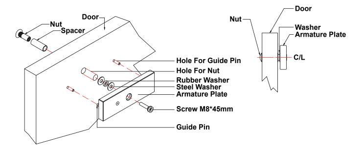
**★★Important**: Fix the armature plate not too tightly,and make the rubber washer more flexible, in order to make the armature plate automatically adjust its proper position with the magnet.
