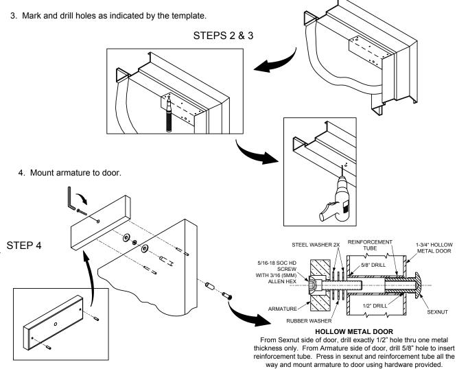
Install mounting plate to header with the interlock detail away from the door side of the stop. Loosely fasten screws through adjustment slot as shown. Assure that the mounting plate and armature line up properly, then tighten down <u>ALL</u> mounting screws.
