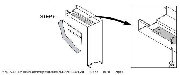
6. Holding the magnet housing at each end, engage the entire length of the interlock detail, by pushing towards the door. Tap with a soft hammer to ensure proper alignment and engagement.
